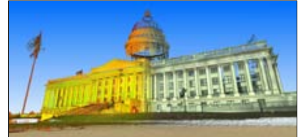
FRONT VIEW OF CAPITOL BUILDING. THE COLORS ON THE RIGHT ARE DERIVED FROM THE PHOTOGRAPHY AND THE COLORS ON THE LEFT ARE FROM THE INTENSITY VALUES THE SCANNER MEASURED.
