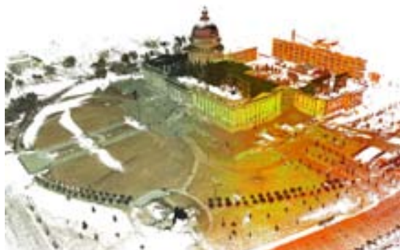
REGISTERED POINT CLOUD VIEW FROM ABOVE. THE COLORS ON THE LEFT ARE DERIVED FROM THE PHOTOGRAPHY AND THE COLORS ON THE RIGHT ARE FROM THE INTENSITY VALUES THE SCANNER MEASURED.
