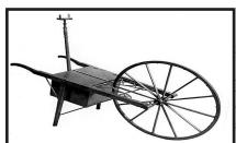
An early distance-measuring wheel used in calculating areas under cultivation.
