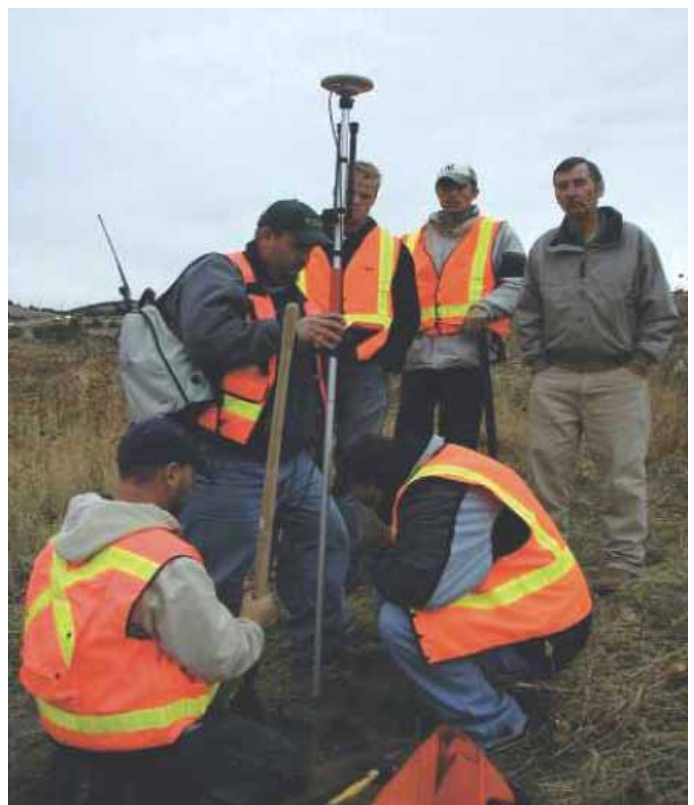
Figure 3. Students setting a section corner using RTK GPS, as part of a 2004 Public Land Surveying Class case study. Richard Green, City Surveyor of Pocatello, Idaho, standing in the back at right.
