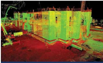
survey. Each mark was checked and then checked again. Also, the pre-cast panels were designed to precisely fit over the many windows of the structure. Prefabricated glass panels were installed in these windows. The pre-cast panels and the glass could not be easily or significantly modified onsite. They simply had to fit when they were installed.
