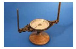
The standard American vernier compass by W. & L.E. Gurley. This form with vernier, outkeeper, sights, level vials, was made from about 1860 and remained in the Gurley catalogs into the 1930s. It attached to either a tripod or Jacobs Staff.
