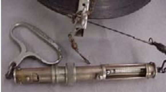
At this point it is worth mentioning a problem that has plagued surveyors using a tape or chain for a couple of centuries - keeping track of the whole lengths that are used when measuring between two points. When a survey crew measured long distances, it is necessary to tally the number of full tape lengths used. Now it would be wise for a crew member to make a mark in a field book each time a tape length is achieved.
