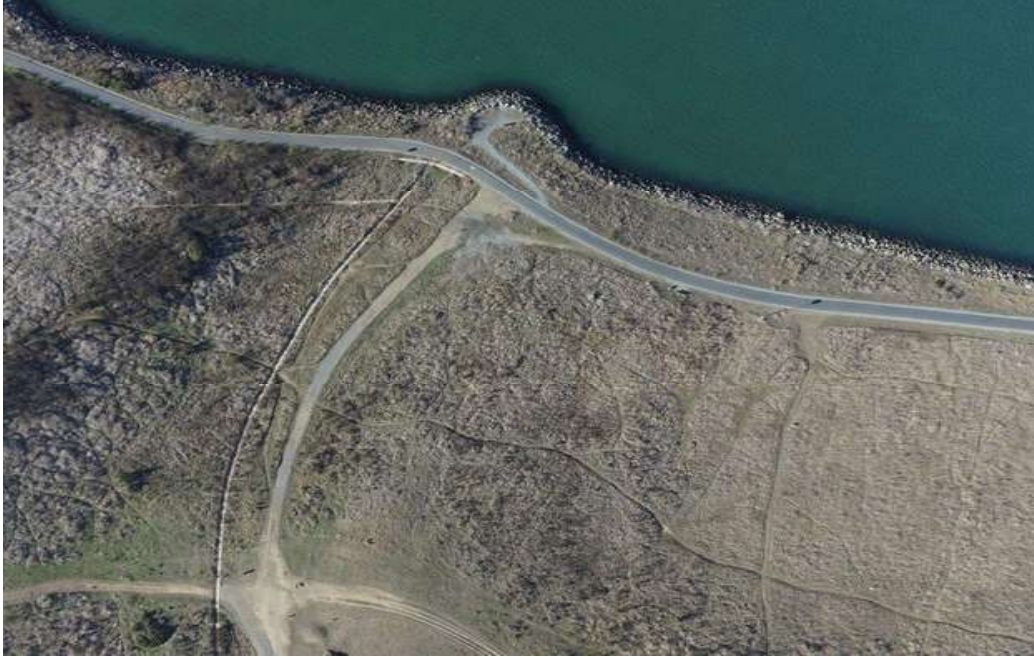
Example of a single nadir image that might be taken during a photogrammetry mission.
